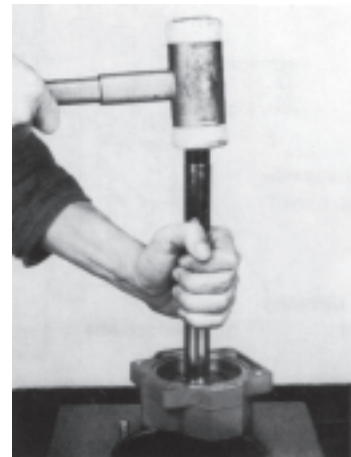
Montage des Wälzlagers (32). Bearing (32) assembly.
