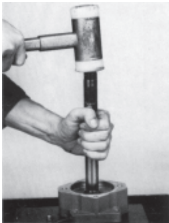
Demontage des Wälzlagers (32). Bearing (32) removal.
